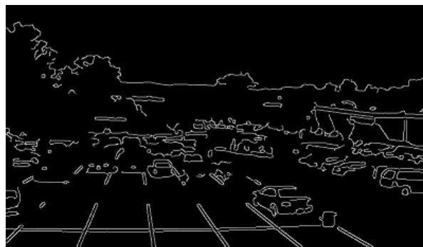
Figure 3. Shows the output from the Canny Edge Detector to automatically allocate available parking spaces and generate ROI
