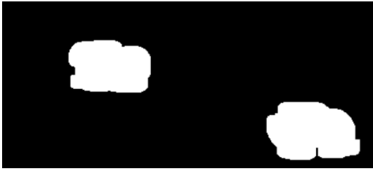
Figure 10. Shows the output after dilation being applied to the image to fill holes in the detected object
