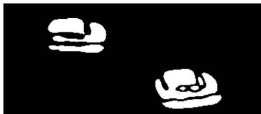
Figure 9. Shows the binary image output after adaptive thresholding being applied to the proposed approach
